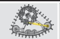
Adjustable pre-loaded spring and multiple rubber dampers keep tracks securely in place and ensure your machine's performance. Our unique system has been improved for better performance and control.
