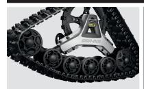
The steel and aluminum frame combines the strength of a traditional steel chassis with a lightweight cast aluminum upper section to offer a lightweight-but-rugged track that can take on any element.
