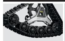
The steel and aluminum frame combines the strength of a traditional steel chassis with a lightweight cast aluminum upper section to offer a lightweight-but-rugged track that can take on any element.
