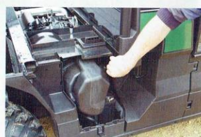
Even with the rear seats in place, the Mule DXT retains a handy amount of room in the rear bay. Sections in the side and rear panels allow a divider to be added, but they also trap dirt and debris.
