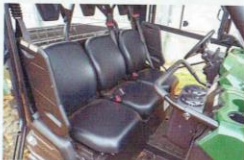
Three separate seats, with some stowage underneath. Though they can get in the way when getting in and out, extended side guards work well with the stubby doors that are fitted to the standard model without a cab. The Viking comes alive across tough terrain.
