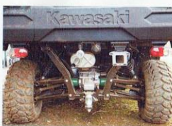
Owners of older Mules will appreciate the independent rear suspension. Less obvious changes are CV as opposed to UJ drivshafts, disc brakes and a proper road-ready lighting kit.
