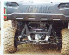
Over-centre clamps lock the rear tailgate firmly in place, the Viking proving able to maintain a fair pace over rough ground in part due to the good suspension set-up.
