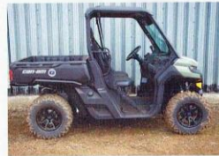
Can-Am Traxter UTV models share essentially the same chassis across HD5, HD8 and HD10 models, these developing 38hp, 50hp and 72hp from their petrol Rotax power units. Respective entry-level prices are £8,583, £10,249 and £14,499.
