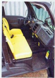
The Gator cab sets a high bar for others to follow, low noise levels enabling easy conversation with a passenger. Heating and ventilation package is hidden in the dash in automotive fashion.
