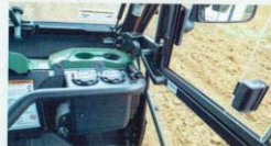
Bolt-on heater pack sits neatly behind removable passenger grab, the latter having finger trapping clearance with the cab door handle.
