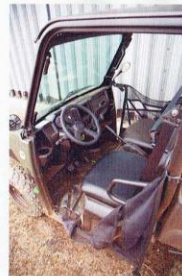
Offering two separate seats, with the parking brake in between, the Ranger provides a comfortable operating environment that appears to be well screwed together. As with other makes and models, net screens and side extensions on the roll-over bar get in the way.
