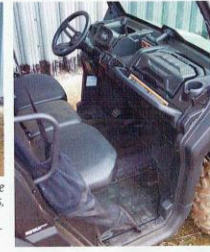
Can-Am Traxter UTV models share essentially the same chassis across HD5, HD8 and HD10 models, these developing 38hp, 50hp and 72hp from their petrol Rotax power units. Respective entry-level prices are £8,583, £10,249 and £14,499.
