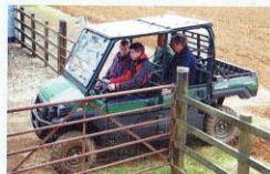
Passengers are well catered for in the Kawasaki Mule Pro DXT, the rear load bay retaining enough space for a bit of load carrying. Folding the rear seats takes a bit of practice, but this version of the Mule is extremely versatile.
