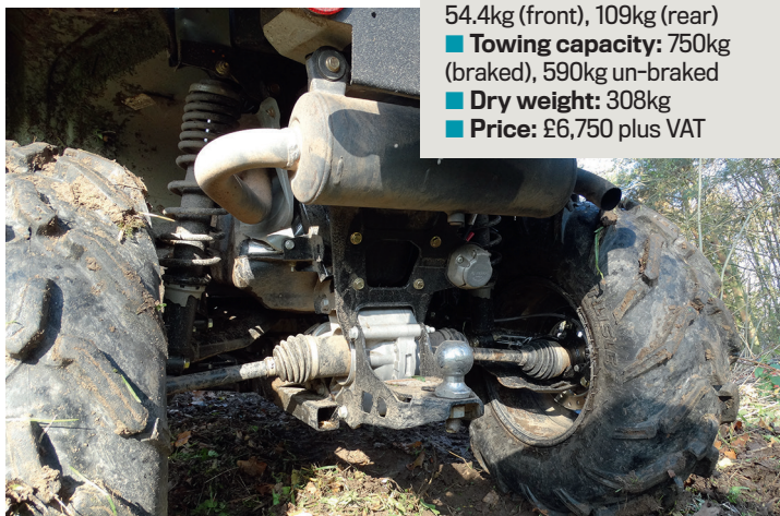
A generous 750kg towing capacity is offered by the 450 Pro T3.
