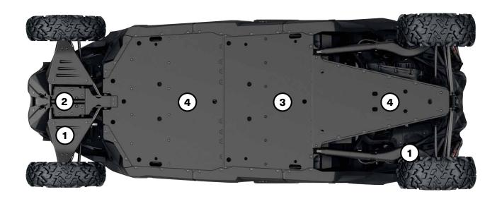
Our plastic plates glide smoothly and silently over obstacles, offering great protection in rough terrain. Made of abrasion-resistant thermoformed 3/8" (10 mm) thick High Molecular Weight Polyethylene (HMWPE).
