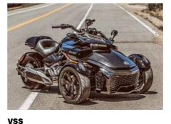
Vehicle Stability System that uses a variety of technologies, including SCS / ABS / TCS, to monitor the vehicle and keep the rider confident on the road.
