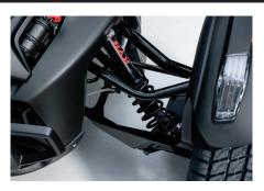
**FULL KYB HPG SHOCKS** Front and rear KYB HPG shocks with remote adjusters and 1 inch of extra suspension travel to optimize your ride and improve comfort.
