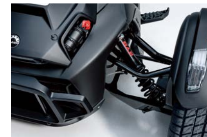
FULL KYB HPG SHOCKS Front and rear KYB HPG shocks with remote adjusters and 1 inch of extra suspension travel to optimize your ride and improve comfort.
