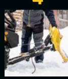
Remove the winch cable from the guide. You're ready to plow.
