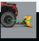
Underbelly mounting plate provides the optimal angle of attack for best push strength.
