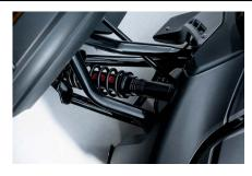
FULL KYB HPG SHOCKS Front and rear KYB HPG shocks with rear remote adjuster for different riding experiences.
