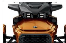
LED HEADLIGHTS The new LED headlamps now offer whiter illumination and a wider periphery, while reducing the amount of maintenance required. Leave nothing hidden with improved road visibility and precision lighting.
